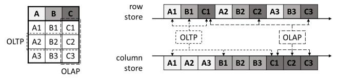
Figure 4: Memory alignment and resulting access patterns for row and column store. Source: own representation based on [2]
